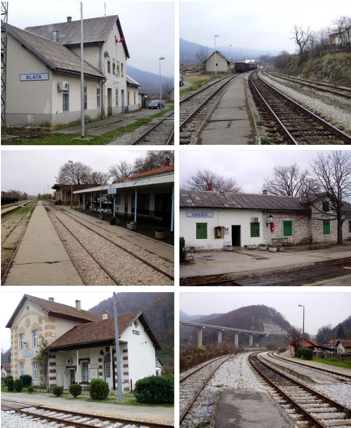
Figure 51: Examples of the security problems at the stations in rural areas Blata, Benkovac, Unešić and Đurmanec (no surveillance systems, lights, unsecure access paths)
